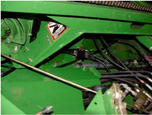
Install hose from outlet 1 of Primary Valve to the inlet of Left Rear Secondary Valve.
