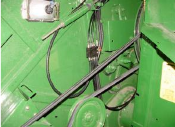
Install hose from outlet 2 of Primary Valve to the inlet of Right Secondary Valve.
