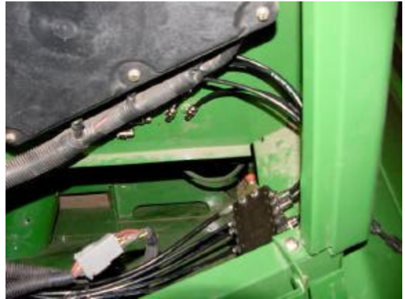
Install hose from outlet 5 of Primary Valve to the inlet of Left front Secondary Valve.
