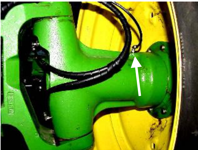
Install one 243699 fitting, replacing grease zerk for Rear Axle Spindle Bearing - Right. Route/install tubing from outlet 9.
