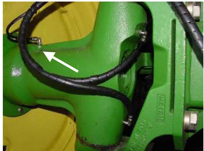
Install one 243699 fitting, replacing grease zerk for Rear Axle Spindle Bearing - Left. Route/install tubing from outlet 10.
