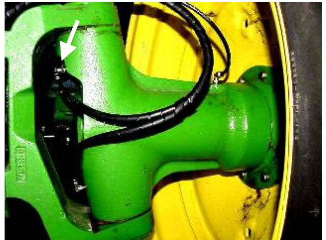
Install one 243699 fitting, replacing grease zerk for Upper Rear Axle Spindle - Right. Route/install tubing from outlet 7.
