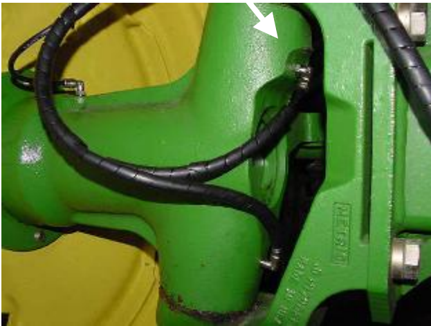
Install one 243699 fitting, replacing grease zerk for Upper Rear Axle Spindle - Left. Route/install tubing from outlet 6.
